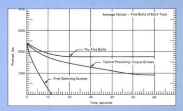
Virtually all threaded bolts are available as Tru-Flex fasteners, including standard size and aerospace fasteners — with various head styles and wrenching recesses. Depending on fastener material, they may be used from -423°F to 1600°F. Maximum temperature for bolts with a plastic locking element is generally limited to 250°F. The Tru-Flex feature does not effect the tensile strength of a bolt.
