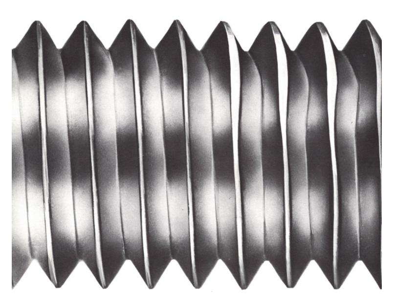
Tru-Flex fasteners are all-metal prevailing torque self locking bolts and screws. The locking action is achieved by a unique thread configuration near the end of the fastener. Tru-Flex screws and bolts are precisely repositioned at the root as well as the crest of at least five threads. This, combined with nonsymmetrical lock location gives Tru-Flex its high performance characteristics of resiliency, reuseability, size accommodation and
