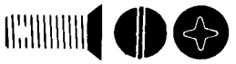
NAS 662 100° Flush Head Self-Locking and Non-Locking, Slotted and Cruciform Recess SPS Jenkintown, Pa.
