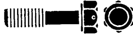
MS 9292 thru MS 9302 Bolt, Hexagon Head, Drilled, 1 Hole, AMS 6322 SPS Jenkintown, Pa.
