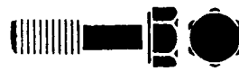
MS 9449 thru MS 9459 Screw, Machine – Steel AMS 6304, Diffused Nickel – Cadmium Plated, Hexagon Head SPS Jenkintown, Pa.
