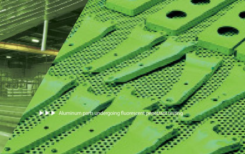
▶▶▶ Aluminum parts undergoing fluorescent penetrant testing
