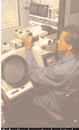
Metallographic sample preparation and examination of optical microscopy verifies proper material processing and fastener manufacturing.
